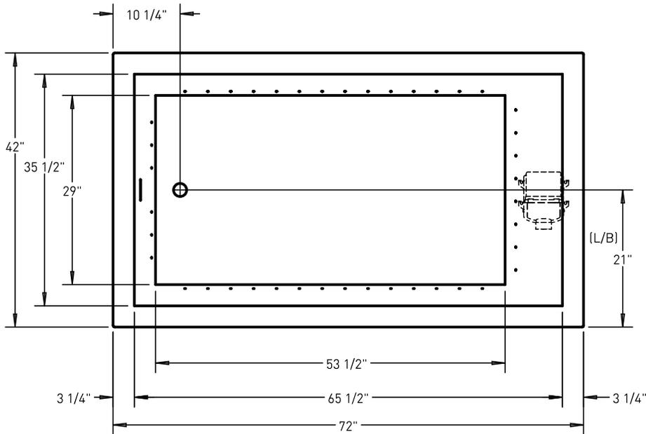
Note: optional pump/blower positions available. R/B for right side drain, L/B for left side drain
