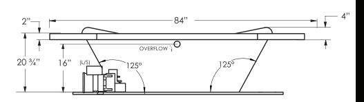
110/115 Volts 20 amp GFI Each pump must be protected by a dedicated GFI breaker (refer to local codes).
